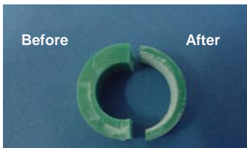
PPR Erosion After 10 months (at 5ppm Chlorine)
